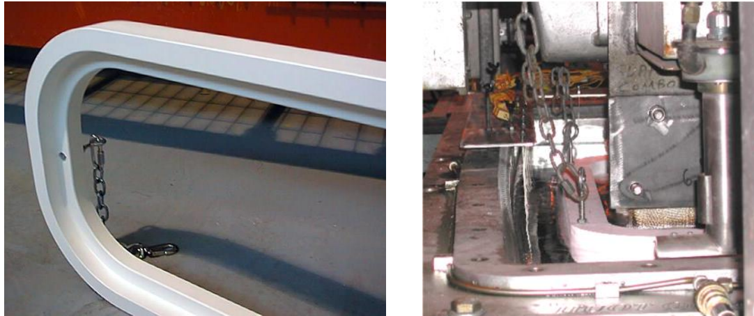
Figure 2. Use of a skim dam during casting. Left: skim dam design, Right: measurement during casting.
